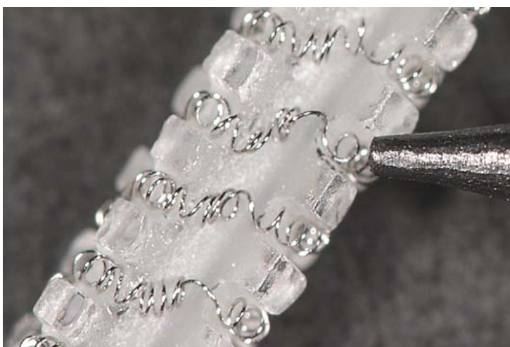
Figure 3 This sensor was probably damaged due to excessive vibration. Notice that many of the coils are shorted together. (The lead pencil is for reference only.)
