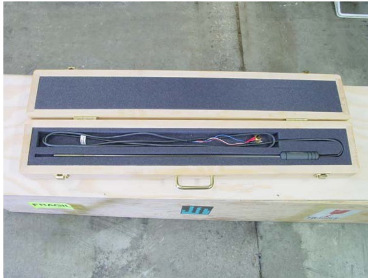
Figure 10 SPRT placed in carrying case
