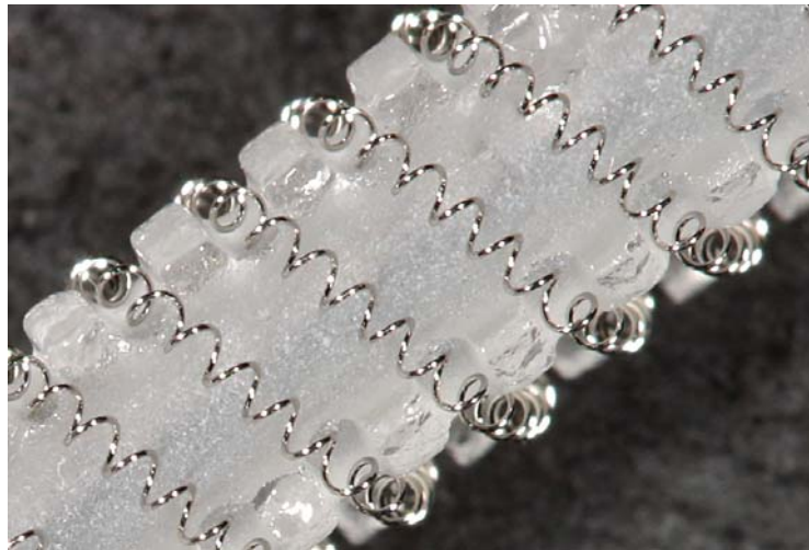
Figure 1 Newly made sensor, note how the coils are very uniform and evenly spaced.
