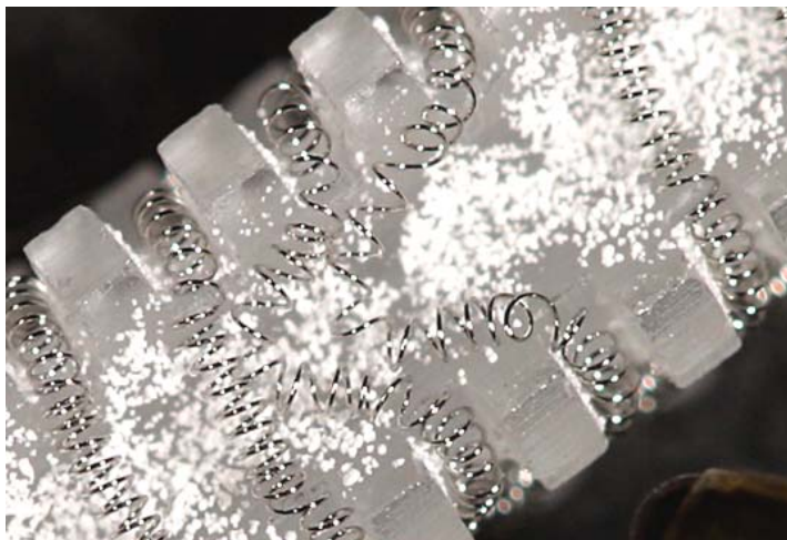
Figure 2 This sensor was probably damaged by acceleration during handling or shipping.
