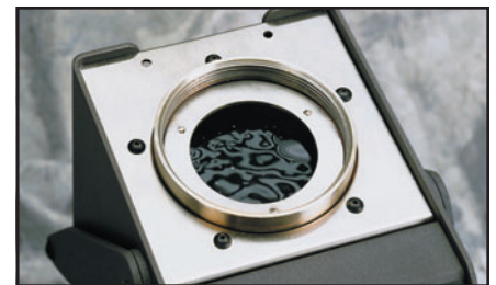
A Micro-Bath's 1.9-inch-diameter tank lets you calibrate just about any size industrial sensor.
