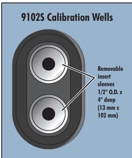
9102S block configuration. Instrument includes 1/4" and 3/16" inserts. Order additional sizes as needed.
